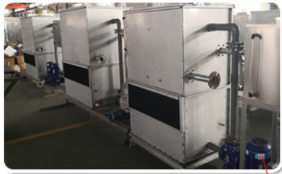
Closed cooling tower
